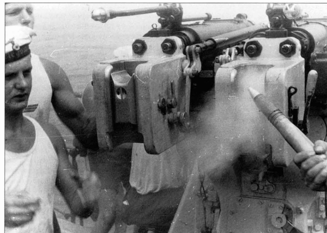
The breech end of what looks like a twin 37-mm quick-firing gun. Shells were fed singly into each barrel. This common calibre has been deduced from the man's hand.
