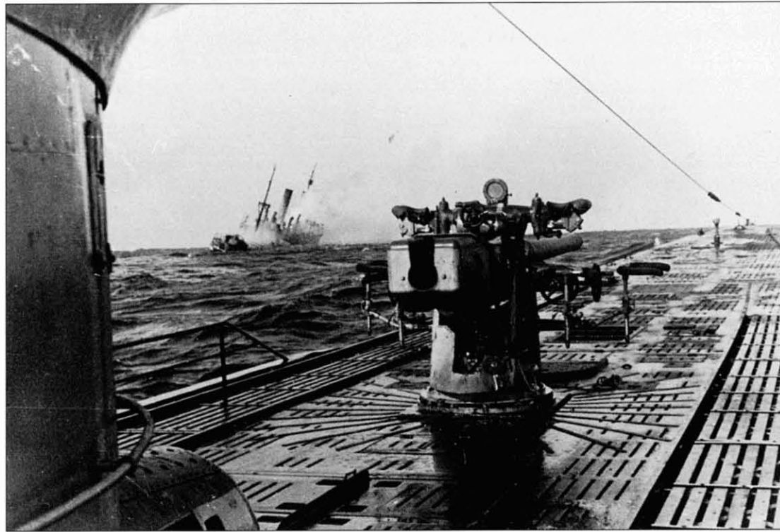
A quick-firing gun aboard U123 , although it looks as if the ship in the distance has been hit by a torpedo. Generally there were two large calibres on U-boats: the wide deck here indicates that U123 was a Type IX, which was usually fitted with a 105-mm gun while the smaller Type VII had an 88-mm weapon.
