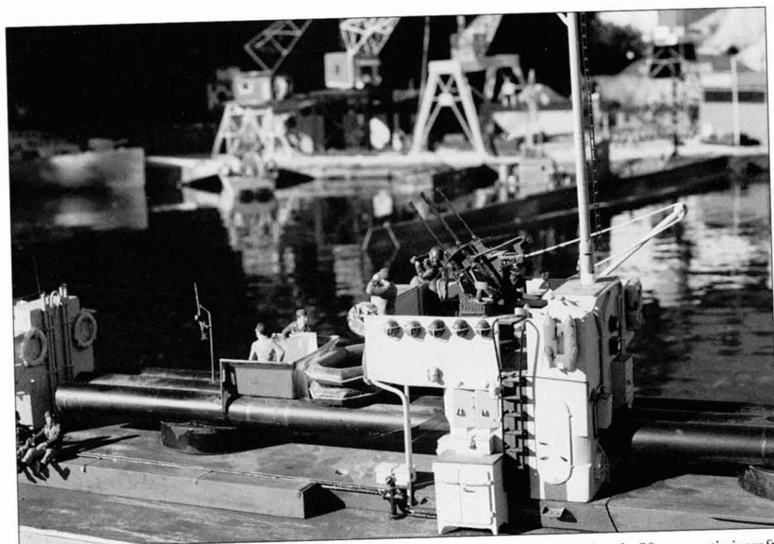
Berntsen's model of T18 , showing the positions of the torpedo tubes and a quadruple 20-mm anti-aircraft gun.
