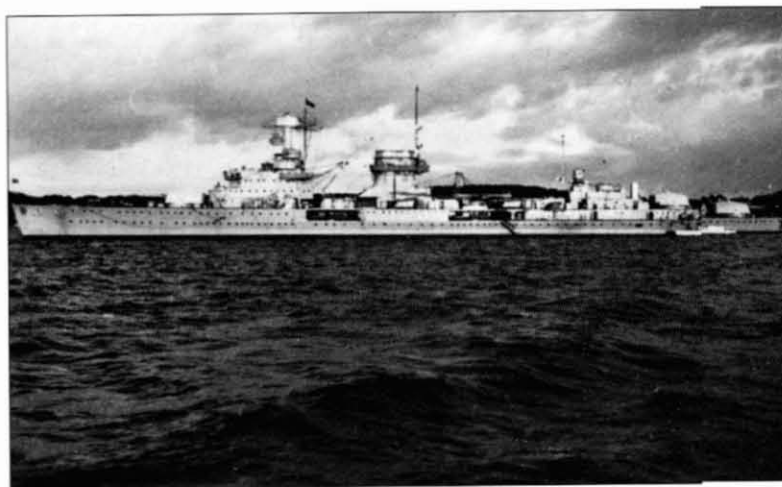
Light cruiser Nürnberg . German designers have helped historians by including a well for torpedo tubes somewhere near the forward funnel. In this case the black box-like feature can be seen between funnel and bridge.
