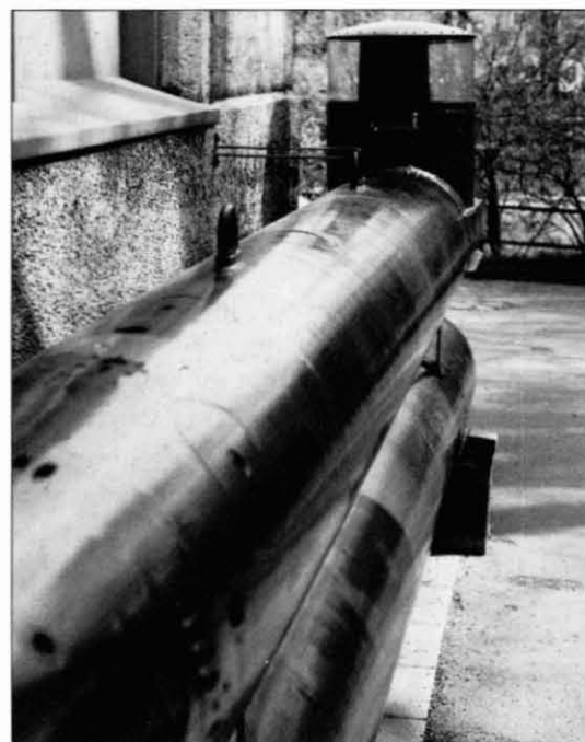
A midget weapon of Type Neger at the Deutsches Museum in Munich (above and below). Although a long way from the coast, the museum has an interesting naval section which includes the U1 boat from before the First World War, a Seehund and a number of surface craft. The tubular window is a postwar addition. Originally it would have been fitted with a Plexiglas dome.
