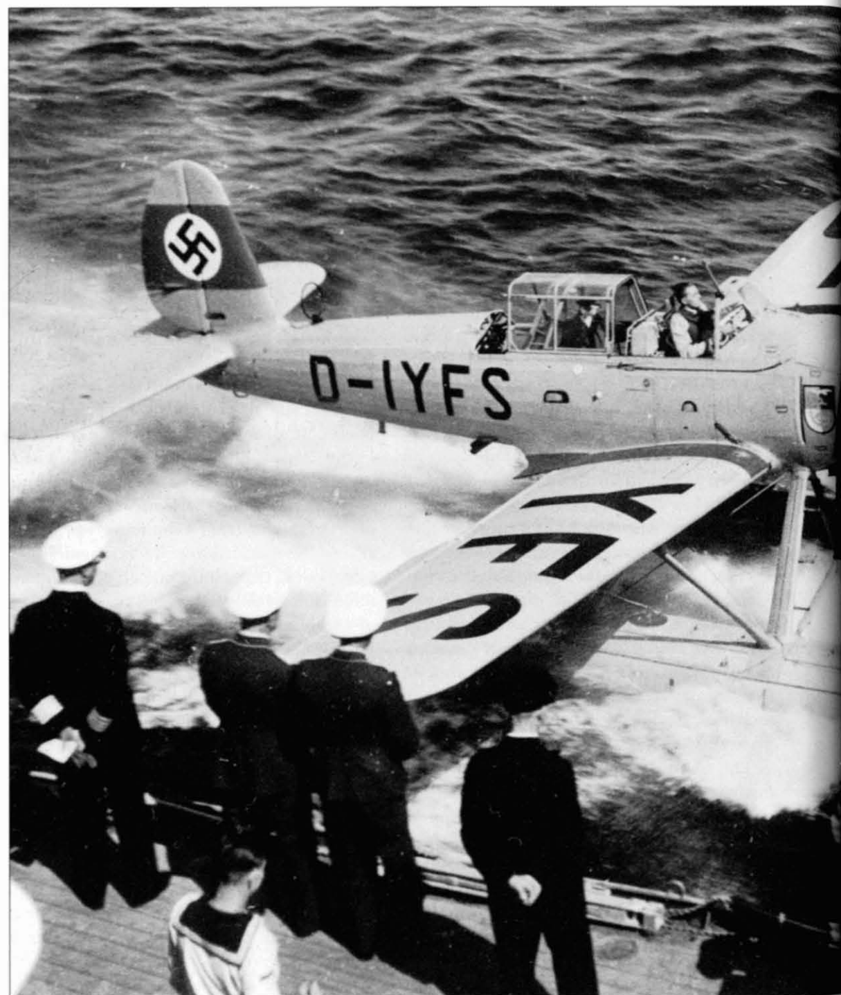
An Arado 196 with civilian registration letters, piloted by Heinfried Ahl of the 1936 Olympia Crew, attempting to land by the side of a warship. The ship, moving at considerable speed, was dragging a heavy rubber mat over the surface of the water with a view to calming the waves. It was found that it was far
