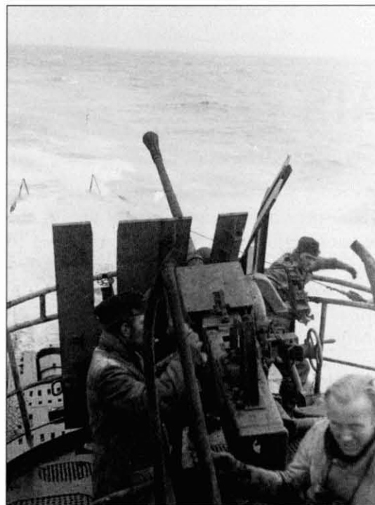
The semi-automatic 37-mm quick-firing anti-aircraft gun aboard U181 under the command of Kpt.z.S. Kurt Friewald. It appears that the weapon is being cleaned because there are no cartridges in the clip above the breech.
