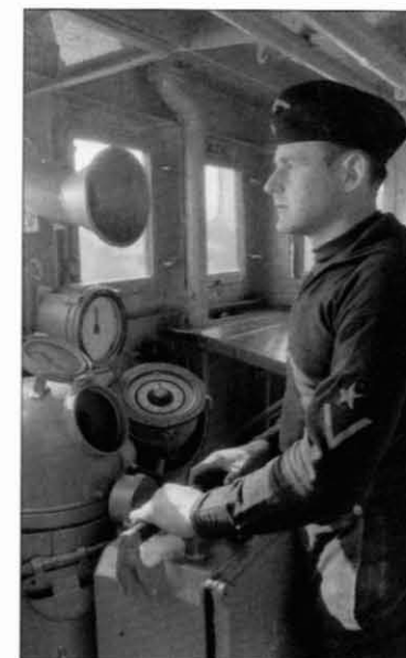
Steering the ship. Below the man's hands are buttons for controlling the electric motor which moves the rudder. In front of him is a speaking tube, a rudder position indicator and gyrocompass. The hood with porthole houses a magnetic compass. The chevron on the man's sleeve indicates his rank of Matrosengefreiter and the star shows that he is a seaman by trade.
