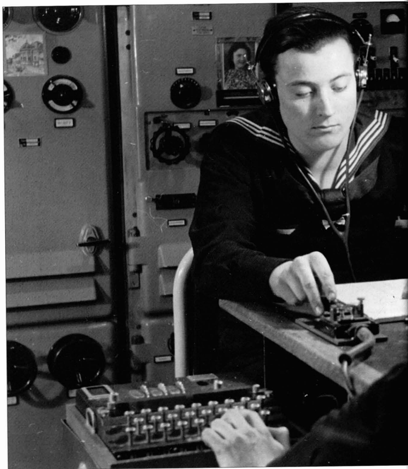
A naval radio room. The typewriter in the bottom left corner, by the man's hand, is a naval version of the famous Enigma code writer. Originally these held three wheels above the keyboard, as can be seen here,
