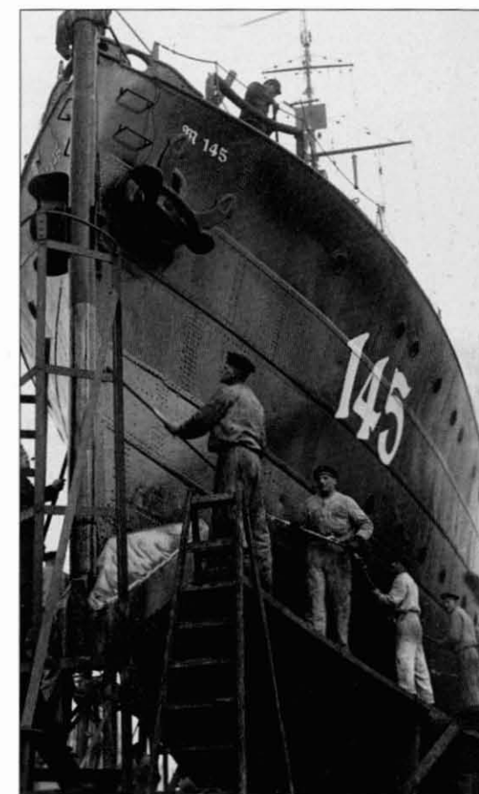
A close up of M145's hull showing the multitude of rivets holding the iron plates together.
