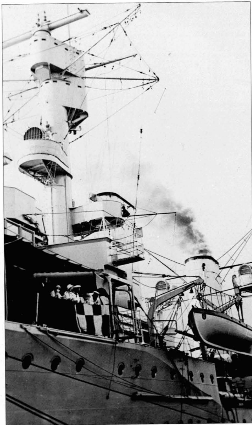
Karlsruhe's main artillery control centre with 10-metre-long optical rangefinder situated at the top of a high tower which also supported a spider's web of radio aerials.
