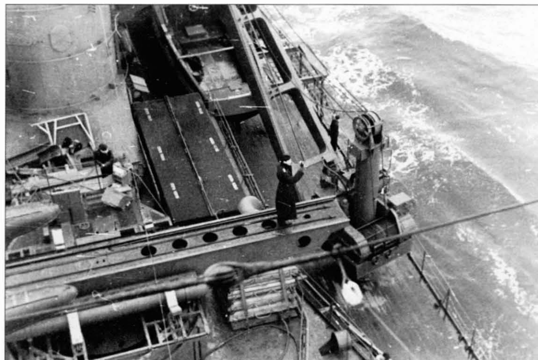
The front of Prinz Eugen 's aircraft catapult with a crane on the deck below. The black roof of the superstructure between the crane and funnel was used to store one of the ship's launches.
