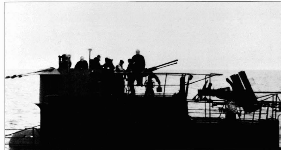
U307 under Oblt.z.S. Friedrich-Georg Herrle showing how anti-aircraft guns dominated conning towers towards the end of the war. In this case there appears to be one double 20-mm on the upper platform, and a 37-mm quick-firing gun on the lower wintergarten . Many boats were fitted with a quadruple 20-mm weapon on the lower platform and two 20-mm twins on the upper.
