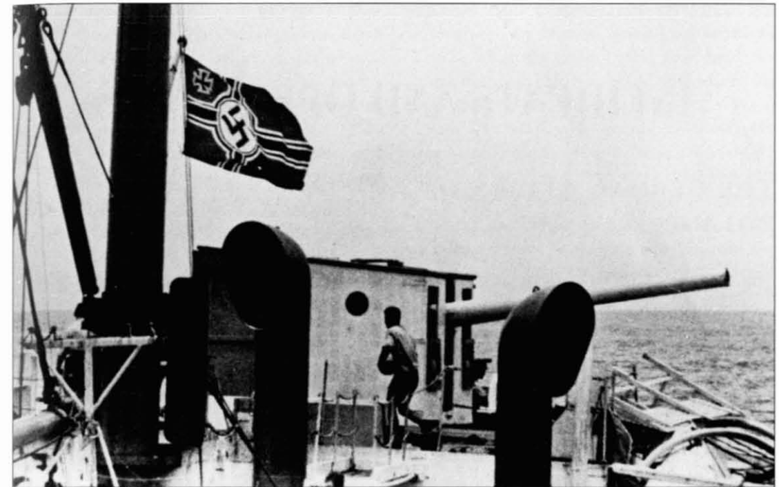
The German war flag flying aboard auxiliary cruiser Widder , with the rear gun uncovered for action. When not in use this was made to look like a deck cabin, hence a bullseye has been painted on the side.
