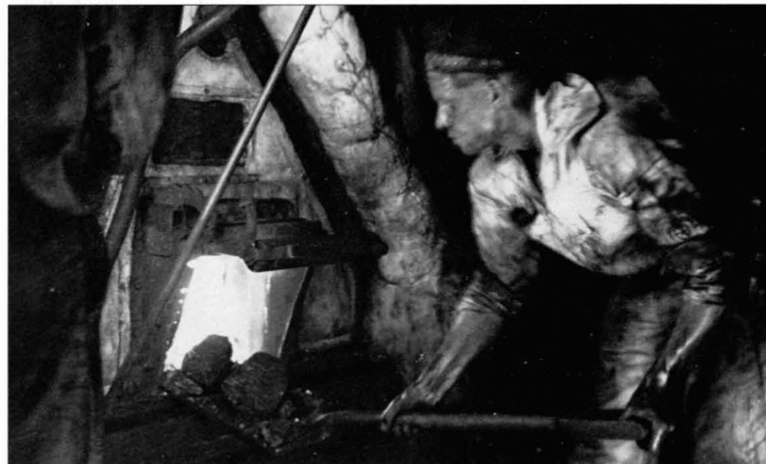
The coal-burning furnaces aboard one of the minesweepers. This filthy work was essential because without it there was no power for anything else.
