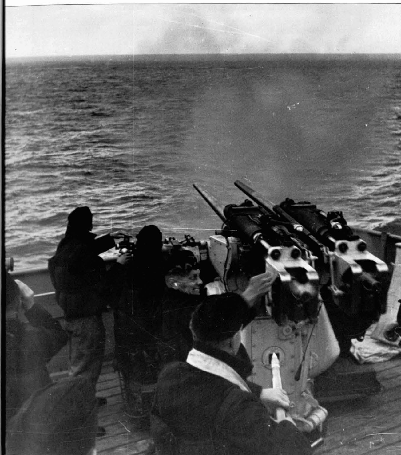
37-mm quick-firing guns in action against aircraft. In this case barrels had to be loaded manually, but the anti-aircraft gun version of this calibre had a hopper for holding a number of shells for more rapid fire.
