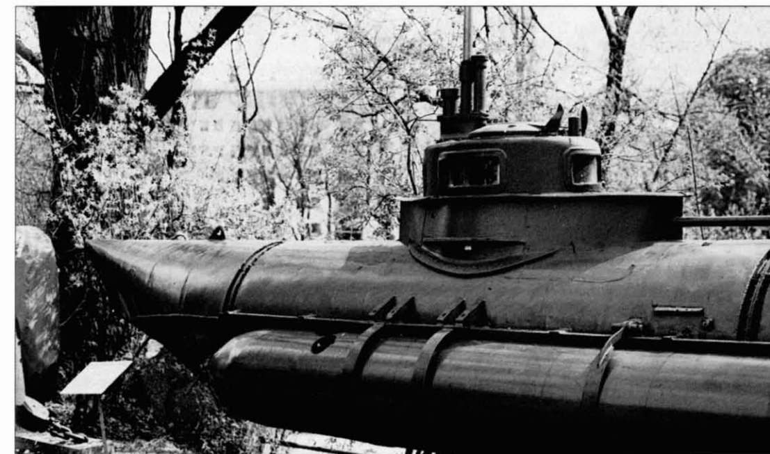
A one-man submarine of Type Biber at the Deutsches Museum in Munich, showing the conning tower and one of the two torpedoes.
