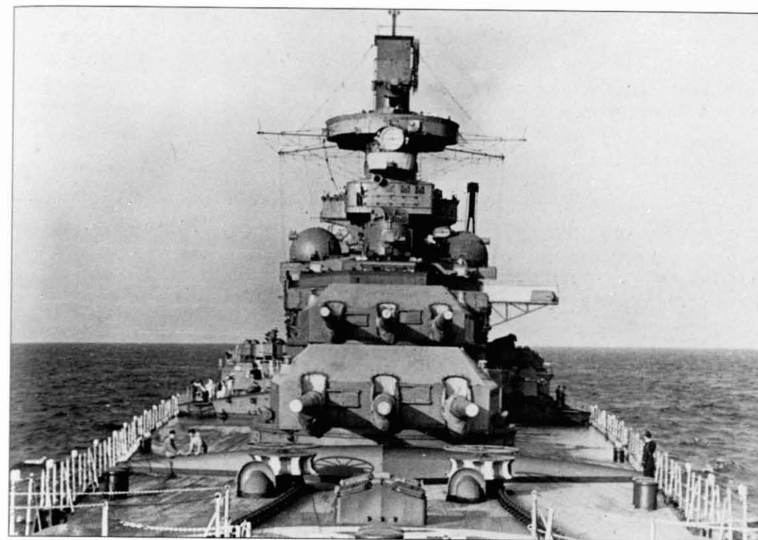
This should be Scharnhorst , although having identified it as such probably means that it is the sister ship Gneisenau because they were so alike. The flimsy extension to the navigation bridge, which can be seen on the port (right hand in the photograph) side suggests that the ship is close to port, because these structures were removed at sea. The rectangular box above the 10-metre-long optical rangefinder is of special interest because a radar aerial has been fitted on the right hand side.
