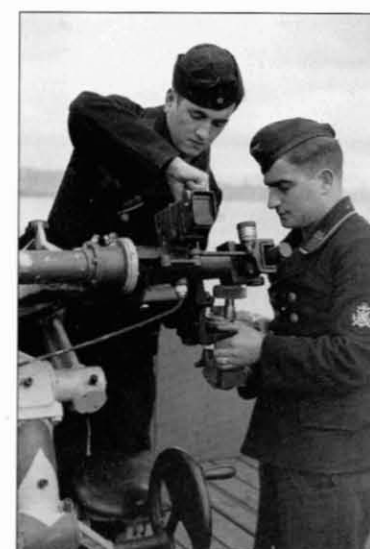
Two naval artillery mechanics adjusting the sights of a 37-mm AA gun. The man on the right is a Maat or petty officer with a distinctive combined rank and trade badge on the left sleeve.
