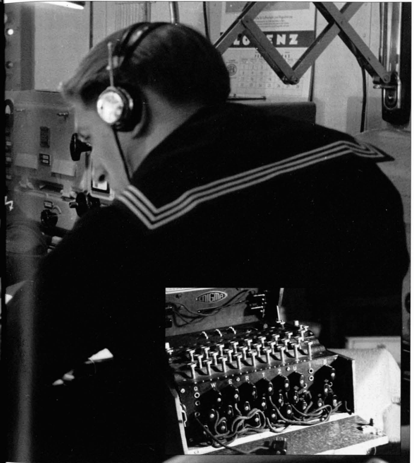
but later the discs were made thinner so that four could be fitted into the same slot. Radio rooms usually also had at least half a dozen different wheels to choose from. Inset: Enigma code writer.
