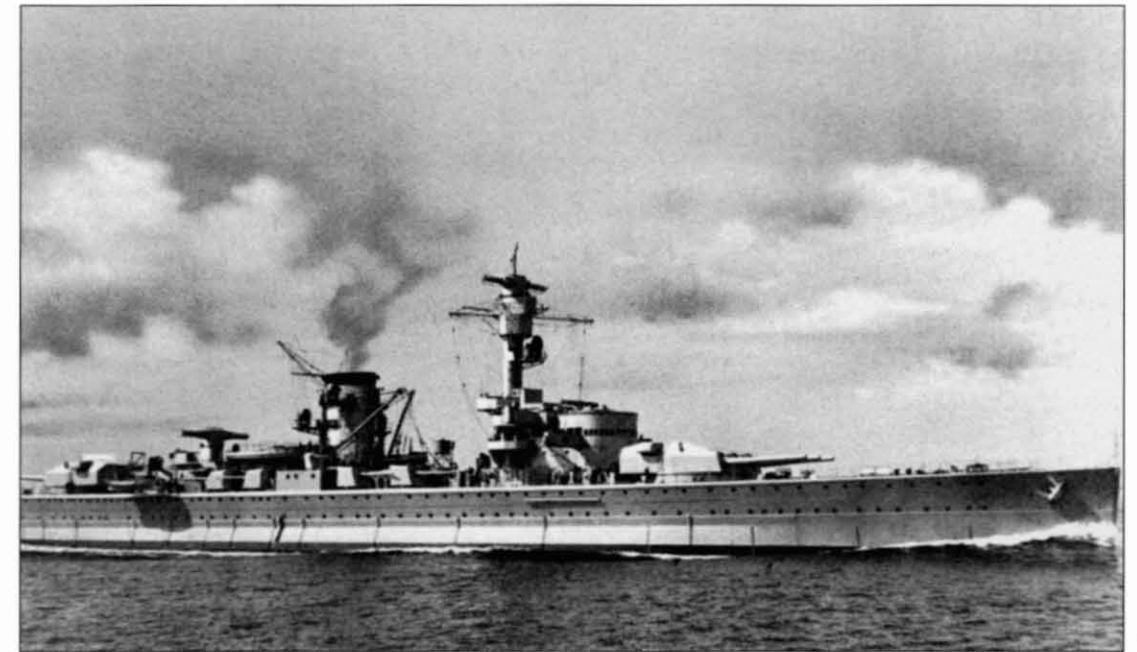
Pocket battleship Deutschland under way. The three main rangefinders can clearly be seen as large 'T'-shaped structures aft of the funnel, on top of the main control tower and on top of the bridge. There were also numerous smaller rangefinders on board.
