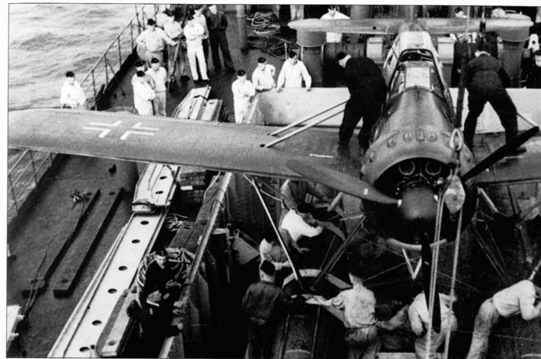
An Arado seaplane being made ready for flight. Wings were removed for storage below decks and the aircraft was hoisted on to the water for take off. This looks very much like a cargo hatch, which would suggest the photograph was taken aboard an auxiliary cruiser. A purpose-built warship would have launched the aircraft from a catapult.
