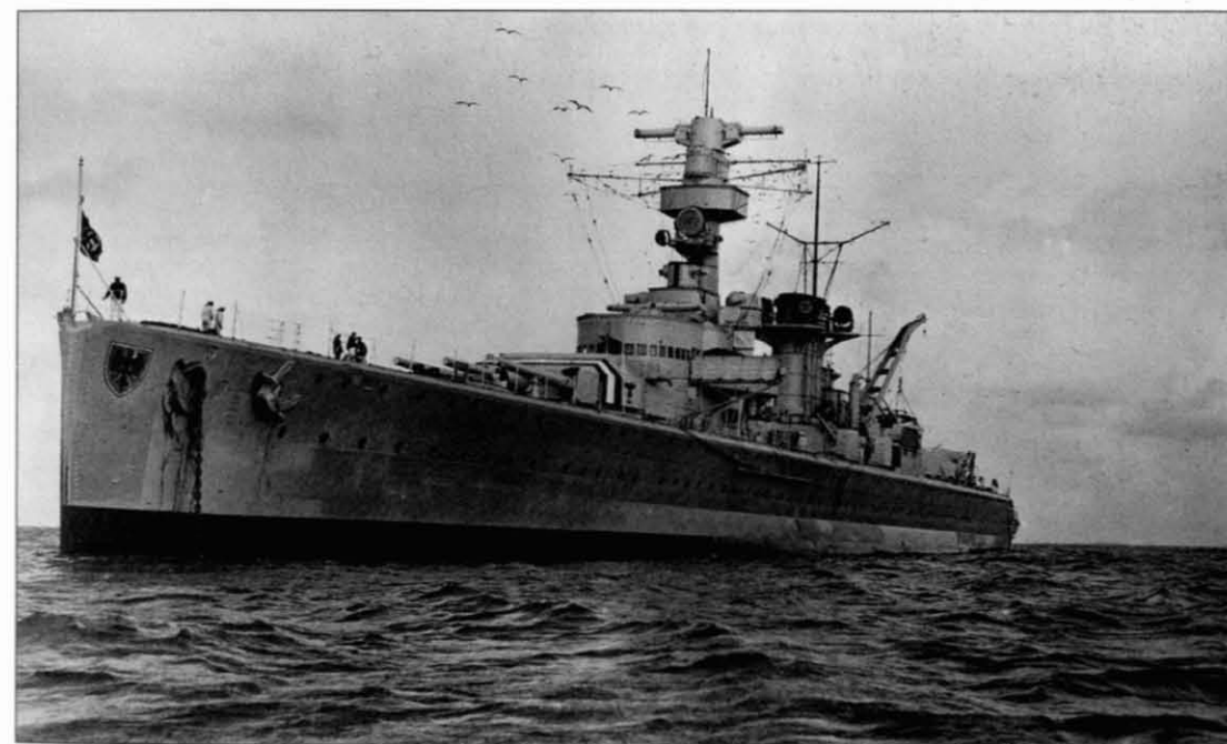
Pocket battleship Deutschland with a red, white and black identification stripe over the forward turret, suggesting this photograph was taken around the time of the Spanish Civil War. The position of the main optical rangefinder at the top of the main control tower shows just how huge these devices were. The quality of the lenses was superb.
