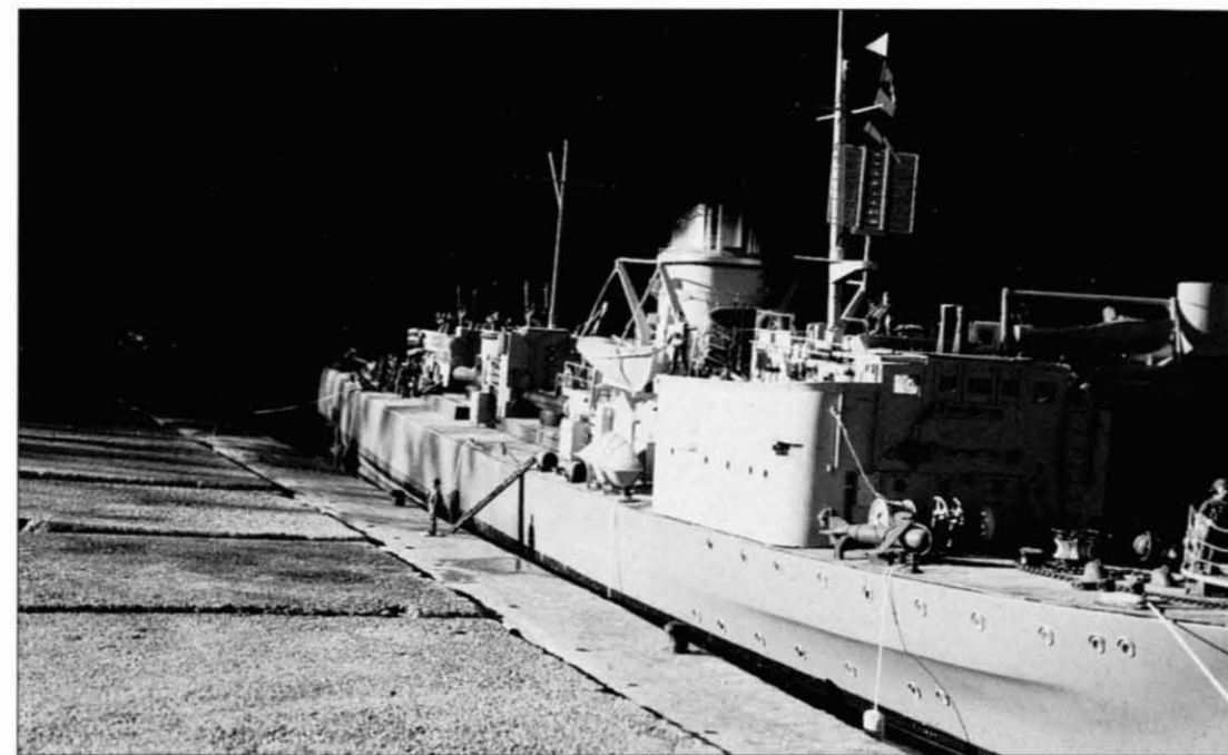
The torpedo boat T18 . Once again a remarkable model by the Norwegian Ivar Bernsten. The paravane, lying on the deck just forward of the bridge, was part of the bow protection gear for clearing mines from the boat's path.
