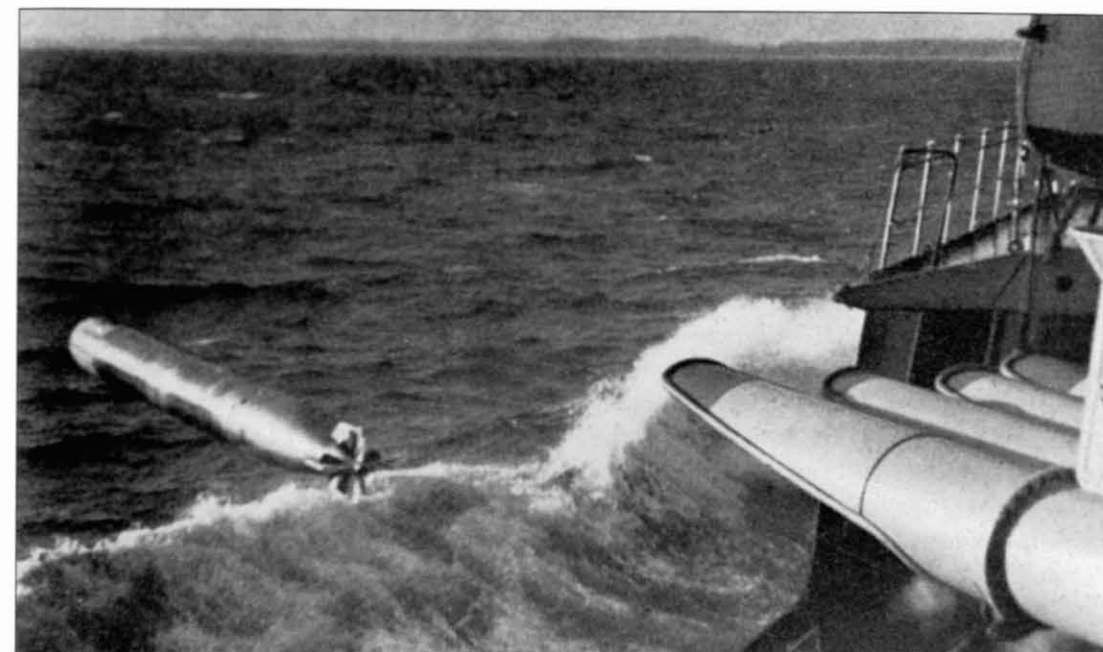
A torpedo being launched. Up to the end of the First World War, the German Navy had experimented with a variety of underwater launching systems, but none of these could cope satisfactorily with ships moving at fast speeds. However, a few of these antiquated systems were installed in auxiliary cruisers during the Second World War.
