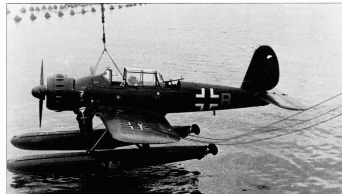
The Arado reconnaissance aircraft from the heavy cruiser Prinz Eugen . Although aircraft could be launched relatively quickly, retrieving them was another problem. They had to land on water, to be hoisted back on board by the nearby crane and this time-consuming procedure could only be carried out in relatively calm weather.
