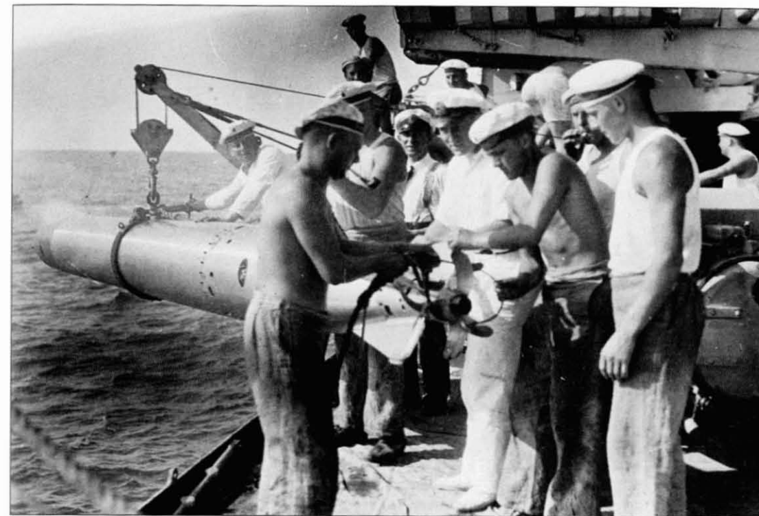
Cadets aboard the light cruiser Karlsruhe practising. Practice torpedoes had a red and white striped head, often with a lamp in the top so that progress could be observed at night.
